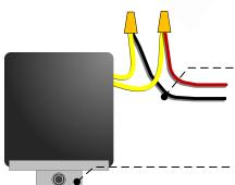
**WIRING USE 18-AWG WIRE TO** CONNECT "COM" & "PC" (CLOSE) TO ZONÈ PANEL
